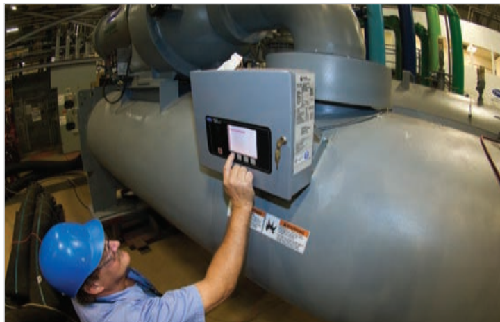
Lab technician Dan Miller performs a final certification test on an Evergreen 19XR water-cooled chiller.
