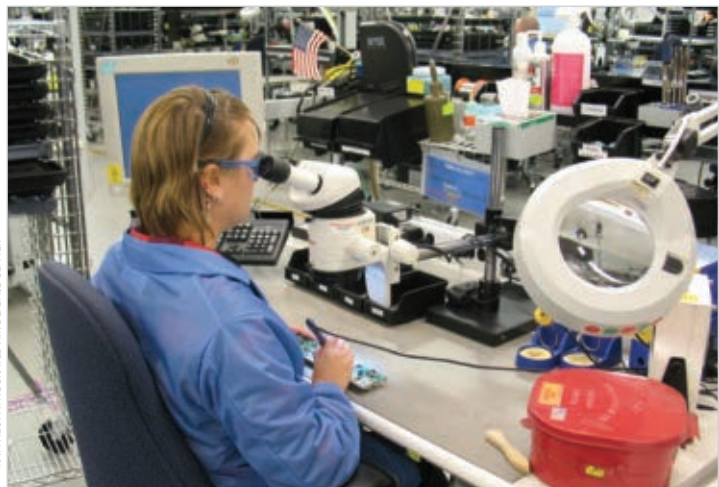
A worker at Raytheon Integrated Air Defense Center's Andover, Mass., facility performs a precision hand solder to a circuit in the circuit card assembly department. The department has achieved a 50% reduction in changeover time over the past three years.
