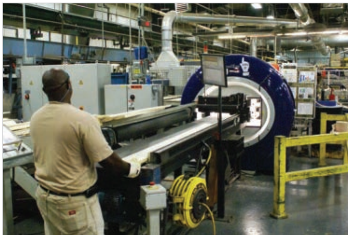
Batesville Casket associate Joe Harris feeds the optimization scanner, which determines the optimal yield for every board it processes.
