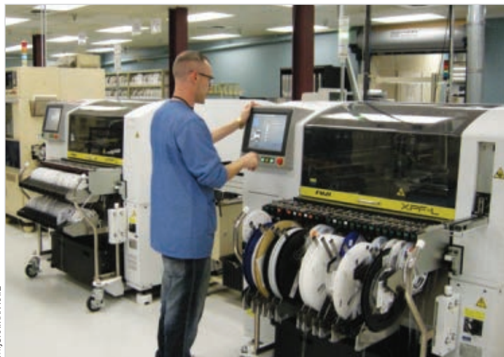
IEC manufacturing operator Kevin Best controls an automated component placement machine. The machine is part of more than $2 million in new-equipment investments in the past three years that have dramatically improved efficiency on the plant floor.
