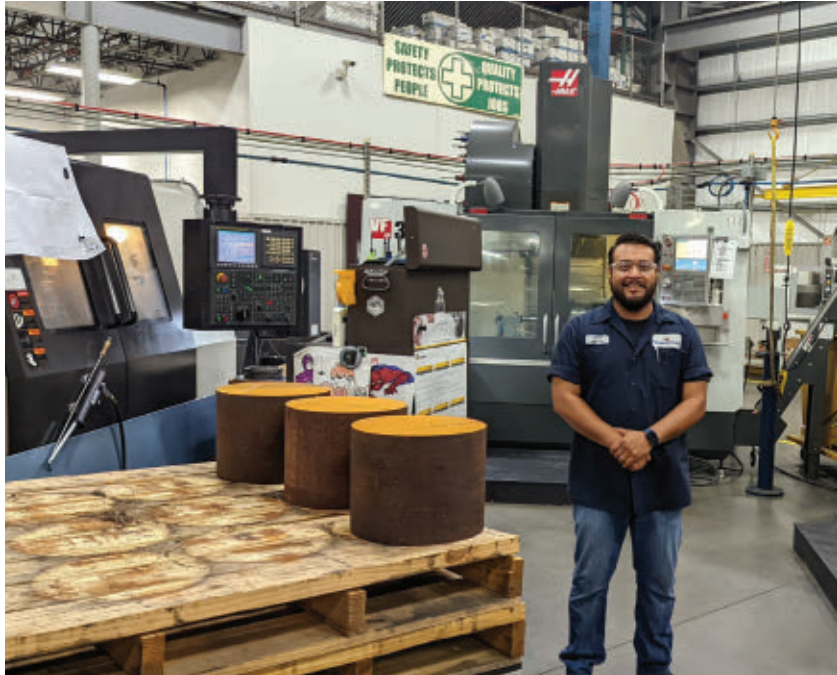
CNC machinist "Super" Mario Perla runs a three-machine cell that produces caps and bonnets used in oil drilling safety equipment. The cell arrangement eliminated excess work in progress. All photos by Robert Schoenberger.
