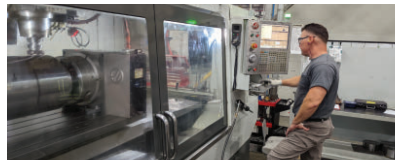
Jose Pesina runs a 5-axis Mori Seiki lathe with machining capabilities. The two-machine cell lowered waste and work-in-process at the plant.
