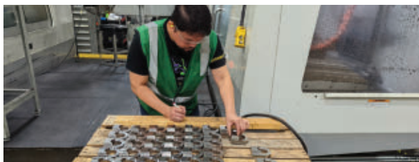
Wilfredo Magbag catalogs ram guides produced in a two-machine cell. Texas Oil Tools uses many forms of color coding—the green vest marks Magbag as a new employee. Orange spray paint on the steel billet notes that it cleared rigorous materials testing.
