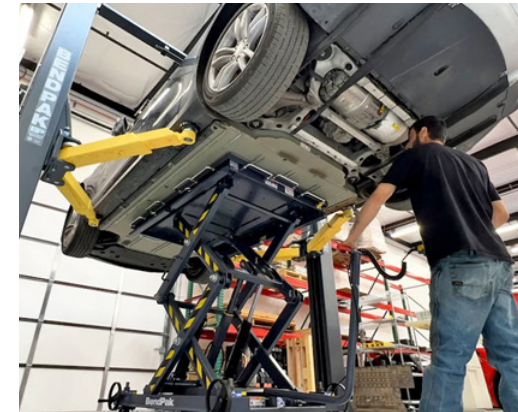
The EV4000SL has a 4,000 lb capacity and the capability to evaluate to more than 6' in less than 20 seconds.
